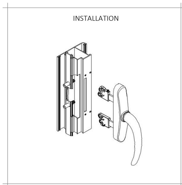
2027 : KEEPER FOR FOLDING SYSTEMS ON OPENING FRAME PROFILE
